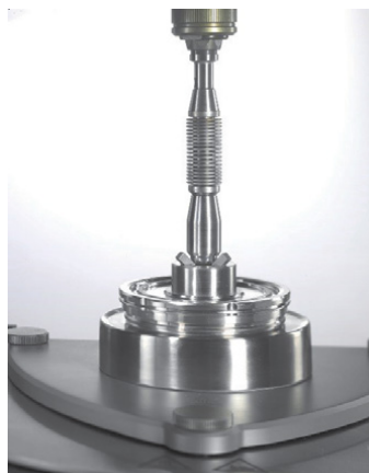
Fig. 2: Tribology setup for HAAKE MARS iQ Rheometer based on the ball-on-3-plates principle.
