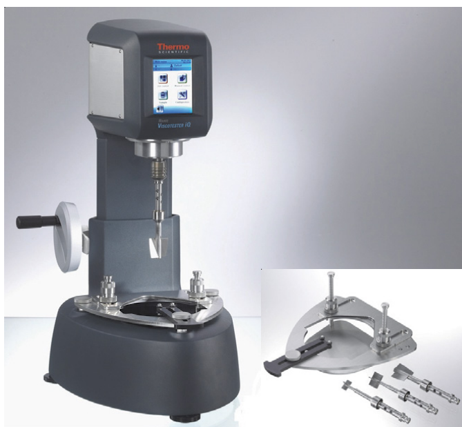
Figure 1: HAAKE Viscotester iQ Rheometer with mounted universal container holder and vane rotor FL26-2 blades (left); universal container holder with three vane rotors: 4-blade rotors FL16 and FL22 as well as FL26-2 blades (right).
