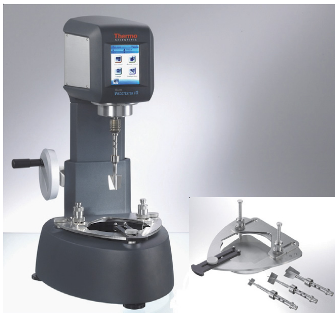
Figure 1: HAAKE Viscotester iQ Rheometer with mounted universal container holder and vane rotor FL26-2 blades (left); universal container holder with three vane rotors: 4-blade rotors FL16 and FL22 as well as FL26-2 blades (right).
