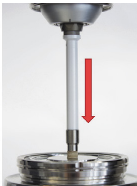
Figure 4: Measurement setup for compression tests using a HAAKE MARS 60 Rheometer and plate-plate geometry P8.
