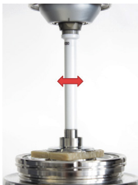
Figure 5: Measurement setup for amplitude and frequency (bulk) using a HAAKE MARS 60 Rheometer and plate-plate geometry P35.
